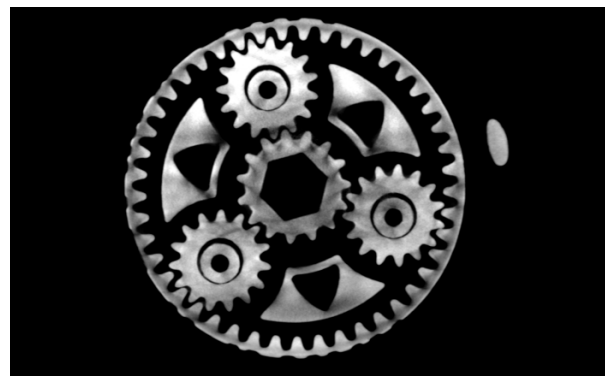
metal printed epicyclic gearing
